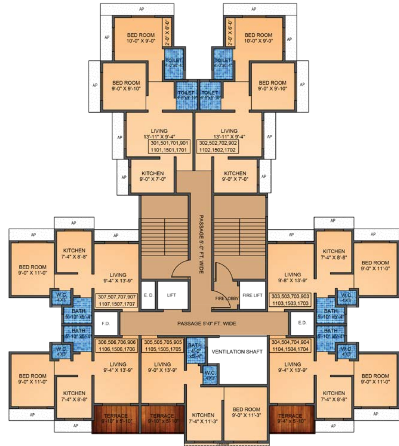
3 RD , 5 TH , 7 TH , 9 TH , 11 TH , 15 TH , 17 TH FLOOR PLAN
