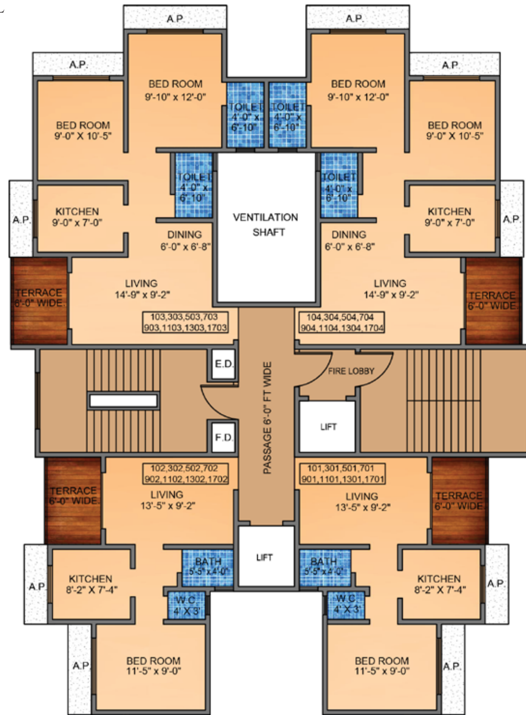
1 ST , 3 RD , 5 TH , 7 TH , 9 TH , 11 TH , 15 TH , 17 TH FLOOR PLAN
